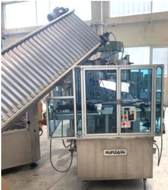
Wirehooding machine NORTAN 8 heads for wirehood 4 wires on glass bottle with long autonomy wirehood store - Nominal output 8.000 bph. Machine set up for three round glass bottle formats
