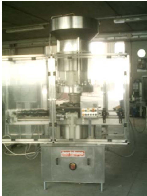
Corking machine BERTOLASO 4 heads for straight cork - Nominal output 6.000 bph. Machine set up for one type of cylindrical glass bottle 75 cl
