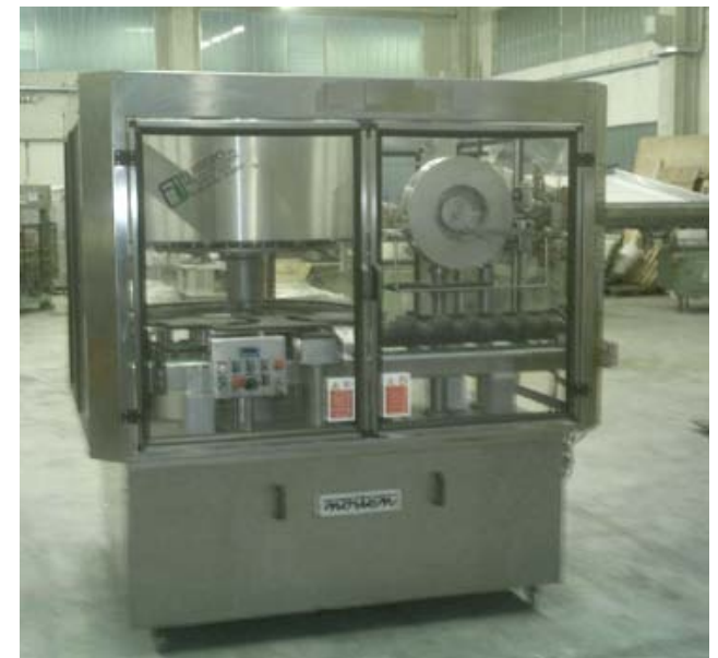
Distributor with thermic heads for PVC capsule - Nominal output 12.000 bph Machine set up for one type of cylindrical glass bottle 75 cl
