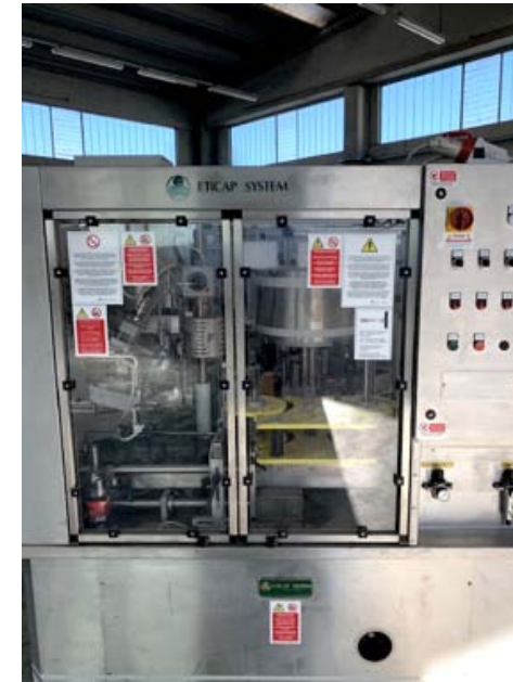
Labelling machine ETICAP , 3-heads, 2 adhesive labeling stations, equipped with: hot foil printer Barban two lanes One bottle change parts 0,75L (yellow colour), One bottle change parts 0,5L (black colour), PVC capsules distributor with thermal head Clockwise running direction
