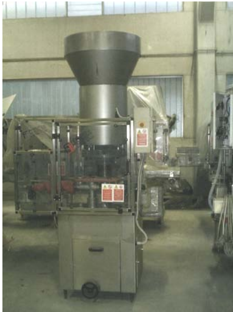
4-head Corking machine AROL, for straight natural cork - Nominal output 6.000 bph. Machine set up for one type of cylindrical glass bottle 75 cl
