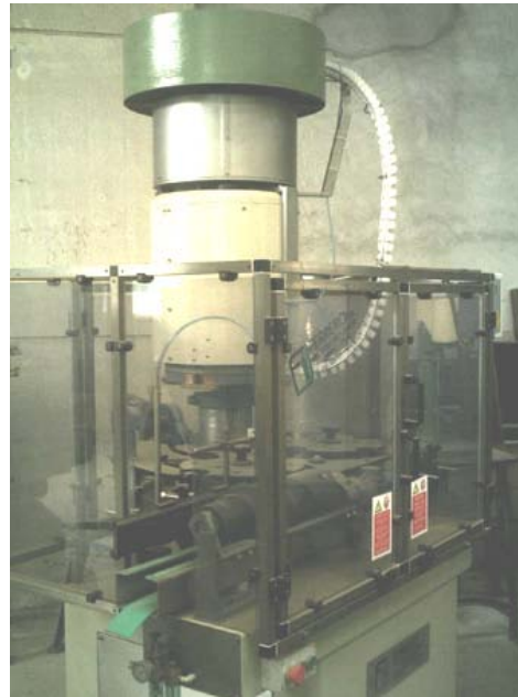
4-head Capping machine BERTOLASO for plastic champagne mushroom cap - Nominal output 6.000 bph. Machine set up for one type of cylindrical glass bottle 75 cl
