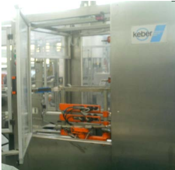
Cartoning Machine KEBER for American carton boxes of 6/12/24 bottles with lower closing by hot melt glue system NORDSON group Nominal output 6.000 bph
