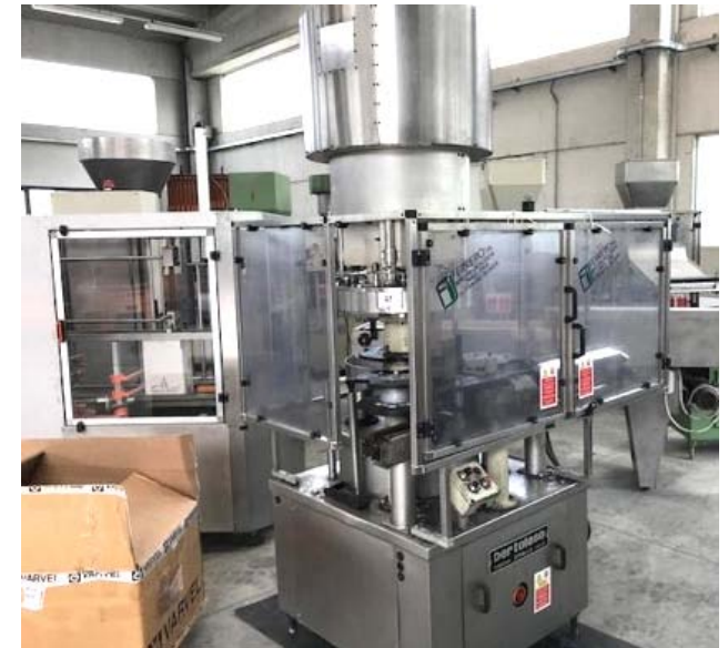
Corking machine BERTOLASO 4 heads for straight cork - Nominal output 6.000 bph. Machine set up for one type of cylindrical glass bottle 75 cl
