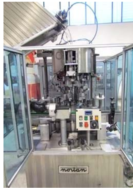
Wirehooding machine NORTAN 8 heads for wirehood 4 wires on glass bottle with long autonomy wirehood store - Nominal output 8.000 bph. Machine set up for three round glass bottle formats
