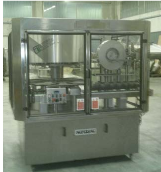
Distributor with thermic heads for PVC capsule Nominal output 12.000 bph Machine set up for one type of cylindrical glass bottle 75 cl
