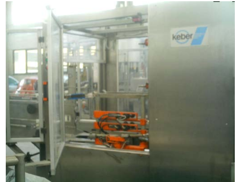
Cartoning Machine KEBER for American carton boxes of 6/12/24 bottles with lower closing by hot melt glue system NORDSON group - Nominal output 6.000 bph
